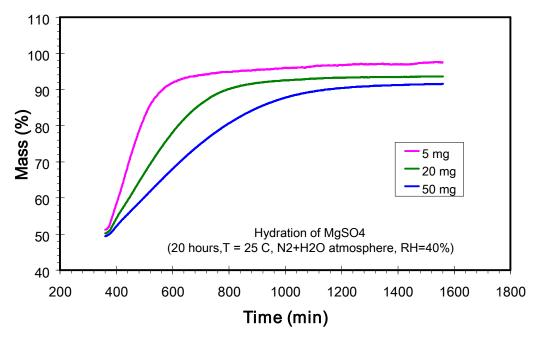
Figure 6: Effect of layer thickness on hydration speed (20 mg corresponds to a layer thickness of roughly 1.5 mm).
