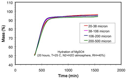
Figure 7: Effect of particle size on hydration.
