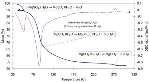
Figure 1: Dehydration of MgSO<sub>4</sub>x7H2O.
