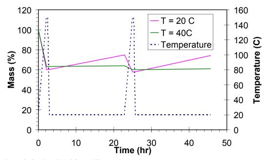
Figure 8: Cycling of MgSO<sub>4</sub> at different temperatures.
