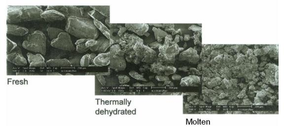
Figure 5: Effect of melting and dehydration on particle structure
