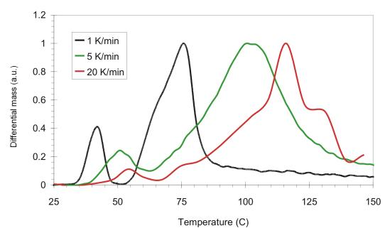
Figure 3: Effect of heating rate on measured dehydration peaks.
