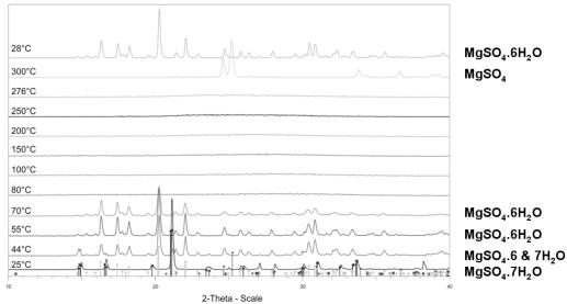
Figure 2: XRD measurements of the dehydration of MgSO<sub>4</sub>x7H2O
