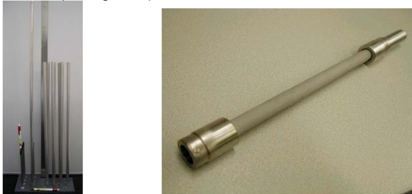
Figure 1 Set of PdAg membrane tubes with a length of 0.6 meter (a) and a membrane with the low cost carbon compression sealing (b)
