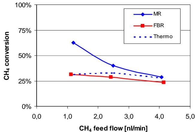
Figure 2 Methane conversion vs feed flow with a membrane reactor (MR), a fixed bed reactor (FBR) and the calculated equilibrium conversion (Thermo) (650°C, 11 bar, feed: CH<sub>4</sub>/H<sub>2</sub>O=1/3).
