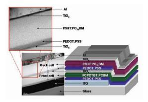
**Figure 1**: The organic multijunction device structure (right) and TEM cross-sectional image (left) of the polymer tandem solar cell [1]
