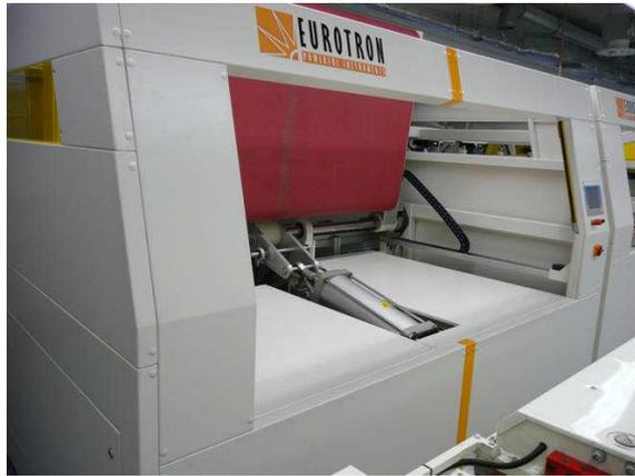
**Figure 8:** Turning unit station that transports the module assembly into a vacuum laminator.
