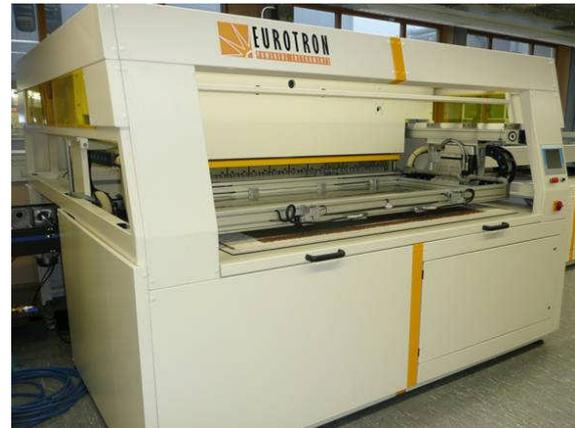
**Figure 6:** Substations for EVA encapsulant lay-down
