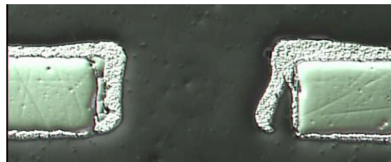
Figure 1: Cracks in the PUM through-hole metallization cause huge fill factor losses.
