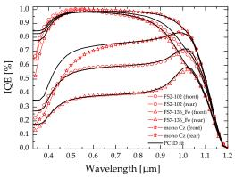
Fig. 5. Internal quantum efficiency for front and rear side illumination of solar cells selected from Cz, reference mc-Si (FS2-102), and a mc-Si ingot with 50 ppmw Fe (FS7-136). The solid lines represent the PC1D calculation, including the fit parameters listed in Table 2.
