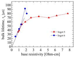
Fig. 4. Minority carrier lifetime in the bulk  $(\tau_b)$  as a function of wafer base resistivity, determined from the PC1D fit of IQE data.
