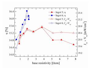
Fig. 2. Experimental power conversion efficiency ( $\eta$ ) and  $J_{sc} \times V_{oc}$  product versus base resistivity of both mc-Si ingots investigated. The record high efficiency of 16.4% is obtained for wafers close to the bottom of ingots 6.
