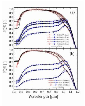
Fig. 3. Internal quantum efficiency for front (empty symbols) and rear side (semi-filled symbols) illumination of solar cells selected from ingot 5 (a) and ingot 6 (b). The legend indicates the wafer's resistivity as well as its position towards the top of the respective ingot. The solid lines represent the PC1D calculation.
