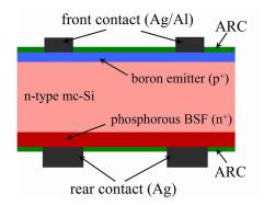
Fig. 1. Schematic cross-section of the n-type solar cell.
