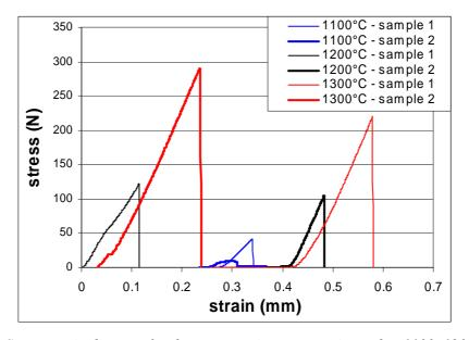
Figure 3.3 Stress-strain diagram for the asymmetric supports sintered at 1100, 1200 and 1300°C.
