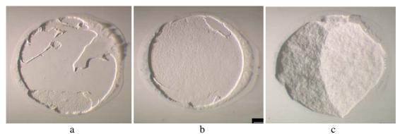
a b c Figure 3.4 Fractography of the fractures surfaces: a,  $1100^{\circ}$ C - interface  $1^{st}$  and  $2^{nd}$  layer,  $b = 1200^{\circ}$ C - interface support tube and  $1^{st}$  layer,  $c = 1300^{\circ}$ C - bulk material support tube
