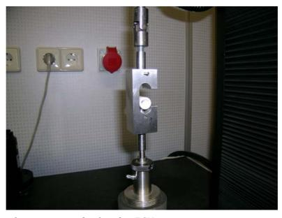
Figure 3.2 Tensile test set up as developed at ECN
