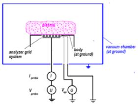
Figure 4: Principle of retarding field analyzer.
