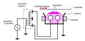
**Figure 2:** Linear RF plasma source for deposition of doped layers in the roll-to-roll system at ECN.
