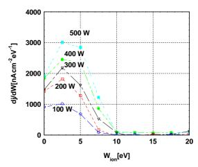
**Figure 7:** Ion energy distribution of the linear radio frequency plasma source versus applied RF-power at 0.1 mbar hydrogen.
