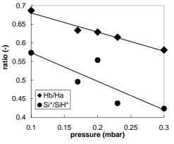
**Figure 8:** Ratio of H $\beta$ /H $\alpha$  and Si\*/SiH\* emission intensities versus operating pressure for H<sub>2</sub>/SiH<sub>4</sub> plasma with a flow ratio of 99. The lines are linear fits to the data.
