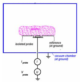
Figure 3: Principle of the Langmuir probe.
