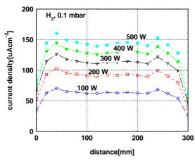
**Figure 5:** Ion density profile of hydrogen plasma generated by the linear RF source at 0.1 mbar as a function of RF power.
