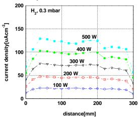
**Figure 6:** Ion density profile of a hydrogen plasma generated by the linear RF source at 0.3 mbar.
