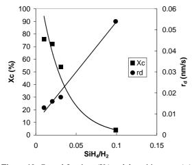
**Figure 10:** Crystal fractions (X<sub>c</sub>) and deposition rates (r<sub>d</sub>) for intrinsic layers grown at various SiH<sub>4</sub>/H<sub>2</sub> ratio's. The trend lines serve as a guide to the eye.
