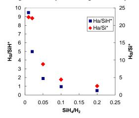
**Figure 9:** Ratios of  $H\alpha/SiH$  and  $H\alpha/Si^*$  emission intensities as a function of  $SiH_4/H_2$  gas flow ratio.
