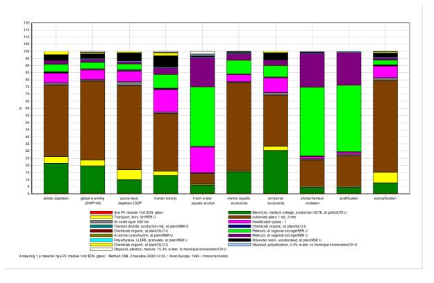
Figure 1: Environmental impact assessment of DSC glass-glass module using CML 2 baseline 2000 method
