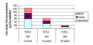
**Figure 3:** Green House Gas emissions of glass-glass DSC modules as function of lifetime (location S-Europe)
