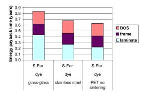
**Figure 2:** Energy payback time in Southern Europe for PV systems using DSC modules with different substrates (8% module efficiency).
