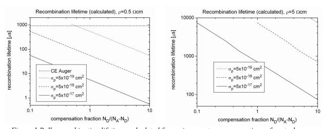
Figure 1.Bulk recombination lifetimes calculated for various capture cross sections of neutral donors. Left:  $0.5~\Omega$ cm resistivity, right:  $5~\Omega$ cm resistivity. Injection level  $10^{14}$  cm<sup>-3</sup>, p-type silicon, donor level Ec-Et=0.045~eV. In the calculation of the compensation fraction, the carrier mobilities are assumed to be unchanged by the compensation. In reality the lines would probably not be straight due to dopant-dopant-interaction.
