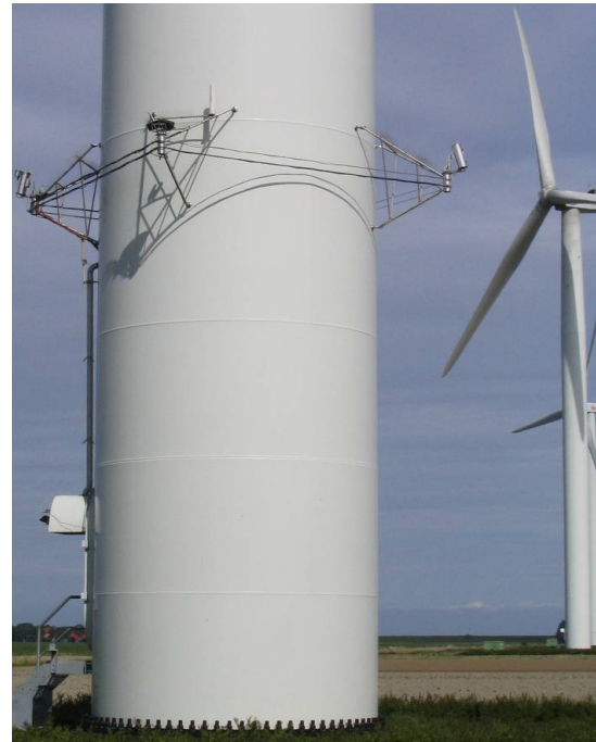
Figure 2: WT-Bird prototype with cameras left and right of the tower and with infrared LED lights and WLAN antennas in front and behind of the tower
