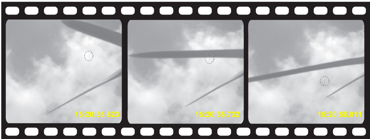
Figure 4: Triggered registration of dummy collision on 20 June 2006.
