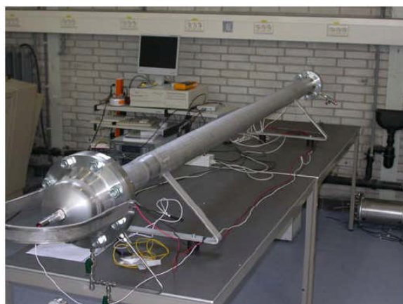
Figure 12 Linear motor driven thermoacoustic cooler.
