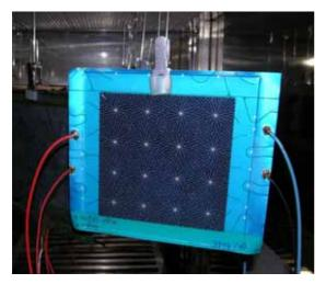
**Figure 2:** Single-cell module in a climate chamber before the test. The connected wires were for measurements in the solar simulator and for power supply in the thermal cycle test. The blue colour of the interconnection foil comes from an isolation coating.
