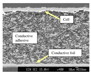
**Figure 3:** Cross-section of an interconnection. The solar cell with silver metallisation pad is visible at the top. The conductive foil is at the bottom. The silver particle distribution in the conductive adhesive is homogeneous and the adherence to both interfaces is good.
