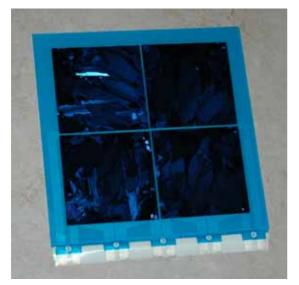
**Figure 6:** Four-cell module with EWT cells. The specially designed back sheet made it possible to flash test the complete module and each cell individually.
