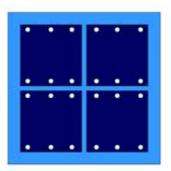
**Figure 5:** Layout of the EWT cells. The dark blue areas are the four cells, the light blue is the interconnection foil and the white points represent the cell contacts.
