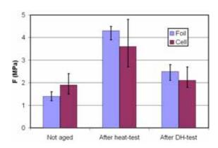
**Figure 1:** Tensile strength results for as-processed buttjoint samples, samples after a heat treatment and after a damp-heat test, either with an interconnection foil interface or with solar cell silver metallisation.
