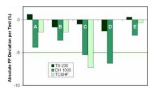
Figure 7: The absolute deviation in fill factor per test for the five four-cell EWT modules. Each module went through a combination of thermal shock, damp heat, thermal cycling and humidity freeze. All modules survived the first three tests. Modules C and D failed during thermal cycling and humidity freeze after thermal shock and damp-heat testing.
