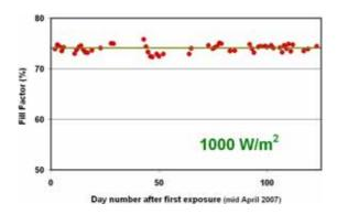
**Figure 9:** The fill factor during outdoor testing of the best performing module remained stable at about 74%. The selected measurements were binned at an irradiance range of 975 to 1025 W/m<sup>2</sup>. The module temperature varied from 25 to 35°C.
