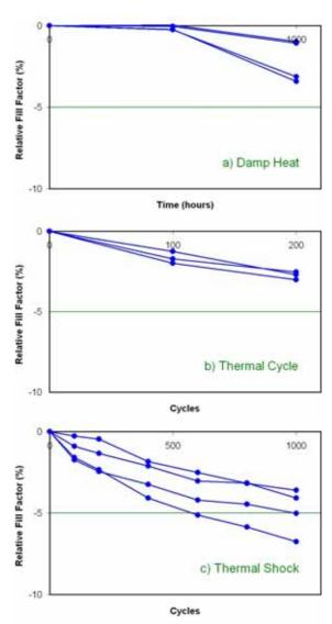
**Figure 4:** The development of fill factor for single cell modules made with a conductive adhesive and interconnection foil during a) damp heat testing, b) thermal cycling at 6.5 A and c) thermal shock testing.
