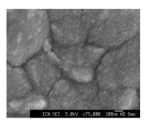
Fig. 4. From left to right: SEM cross section of ZnO:In (A) (x40.000) and cross section (x40.000) and top view (x75.000) of (i-ZnO)/ZnO:In (B)
