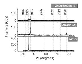
Fig. 5. X-ray diffraction spectra (coupled scan) of i-ZnO, ZnO:ln (A) and (i-ZnO)/ZnO:ln (B)
