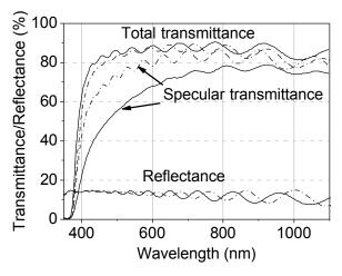
Fig. 6. UV-VIS spectra of ZnO:In (A) (solid lines) and (i-ZnO)/ZnO:In (B) (dash-dotted lines) (The layer thickness is 1300 nm).
