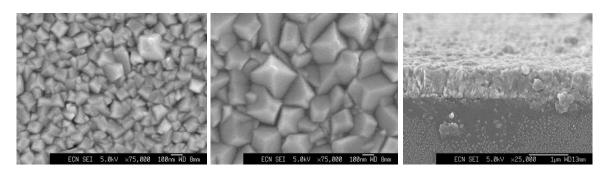
Figure 1 From left to right: SEM top view of a 300 nm thick ITO layer (x75.000) and SEM-top view (x75.000) and cross section (x50.000) of a 800 nm thick ITO layer
