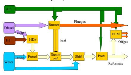
Figure 2. Simplified block diagram 25 kW demonstrator for diesel reforming
