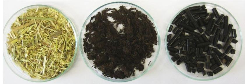
Arundo donax, before and after Torwash ® , and after subsequent pelletization
