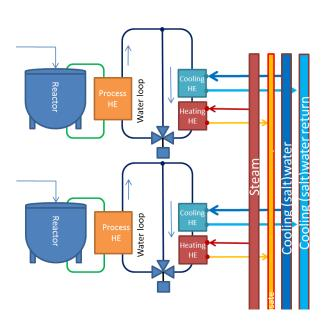
Heat rejection of water loop
