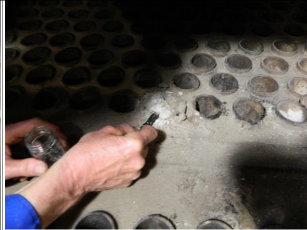
Heavy deposit and sampling, Pipe A12
