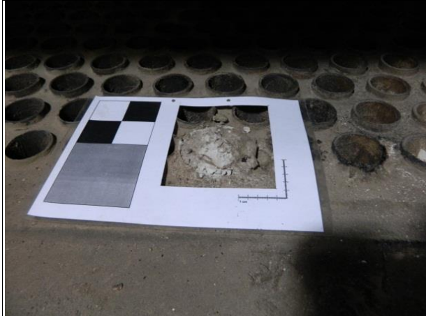
Heavy deposit and sampling, Pipe A12
