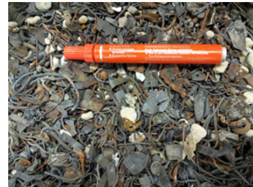
Small pieces of metal, sieved out of bottom ash
