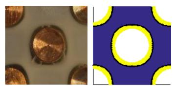
Study of melting behaviour of a PCM storage concept, experiment + model
