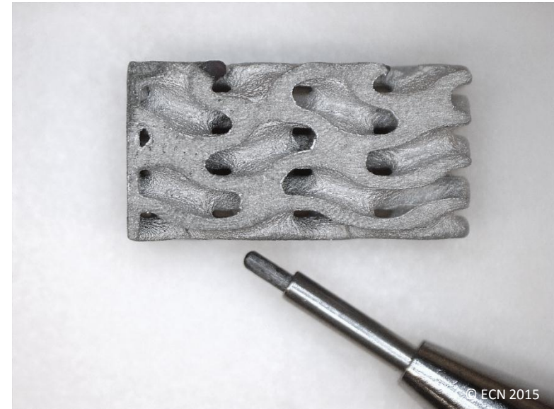
3D printed geometry - sintered
