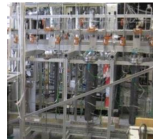
Series of further gas cleaning and methanation
