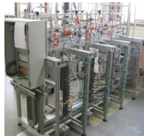
Series of further gas cleaning and methanation
