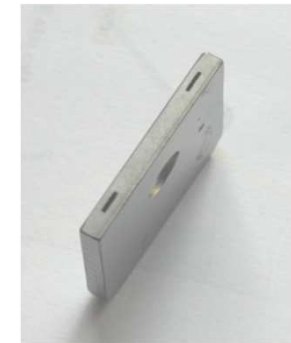
Internal voids e.g. cooling channels possible
