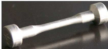
As sintered Standard Tensile test sample
