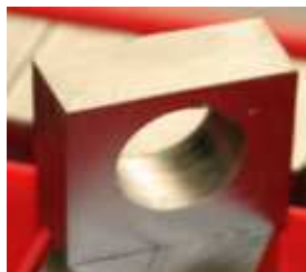
As sintered monoblocks and mock up for ITER divertor target
