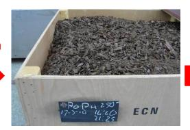
Brittle and less fibrous LHV = 18 - 24 MJ/kg Hydrophobic Preserved Homogeneous
