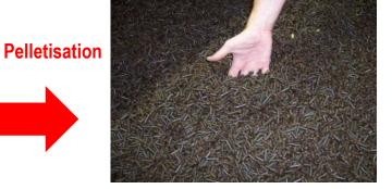
Bulk density 650 - 800 kg/m<sup>3</sup> Bulk energy density 12-19 GJ/m<sup>3</sup>
