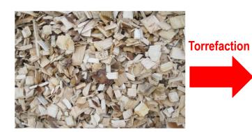
Tough and fibrous LHV = 9 - 12 MJ/kg Hydrophilic Biodegradable Heterogeneous
