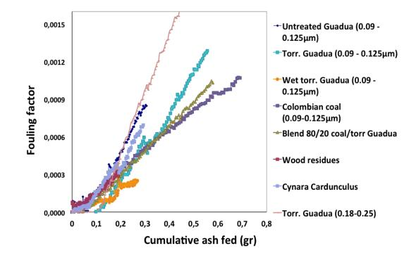
$R_f$  – fouling factor, (K·m<sup>2</sup>)/W (heat transfer resistance)
