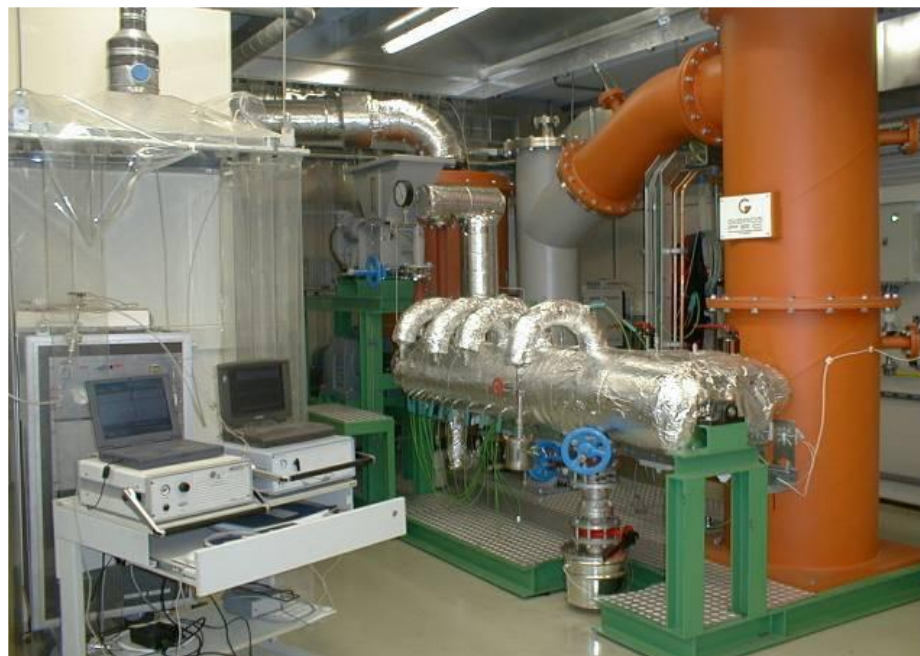
5 kg/h Auger reactor (screw reactor)
