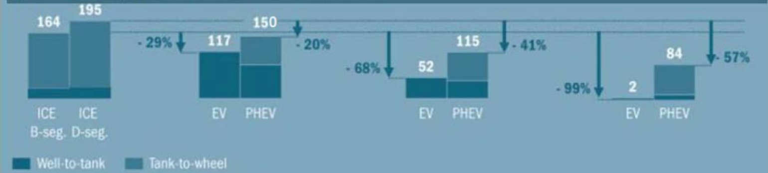
CO 2 emissions of conventional vehicles (ICE) vs. electrical vehicles (EV) and plug-in hybrids (PHEV) (well-to-wheel, g/km, B-seg. = gasoline, D-seg.=diesel) 2)
