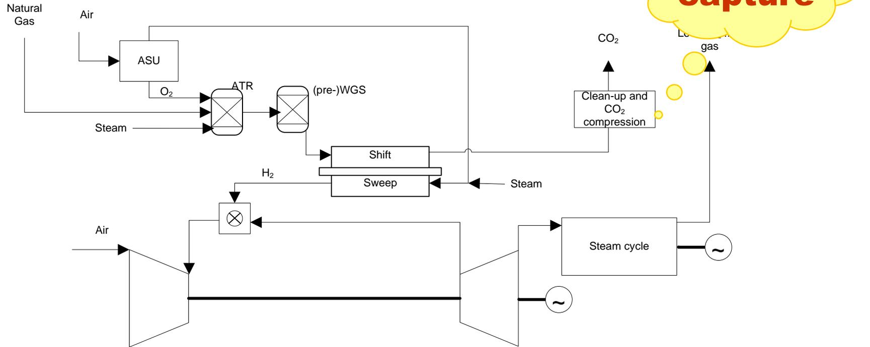
General layout of a power plant with a **membrane water gas shift reactor (M-WGS)**
