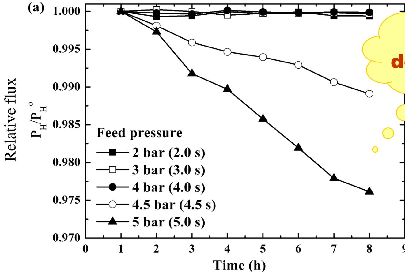
*10% CO<sub>2</sub>/H<sub>2</sub> mixtures at 450 °C and a feed flow rate of 2 NI/min*
