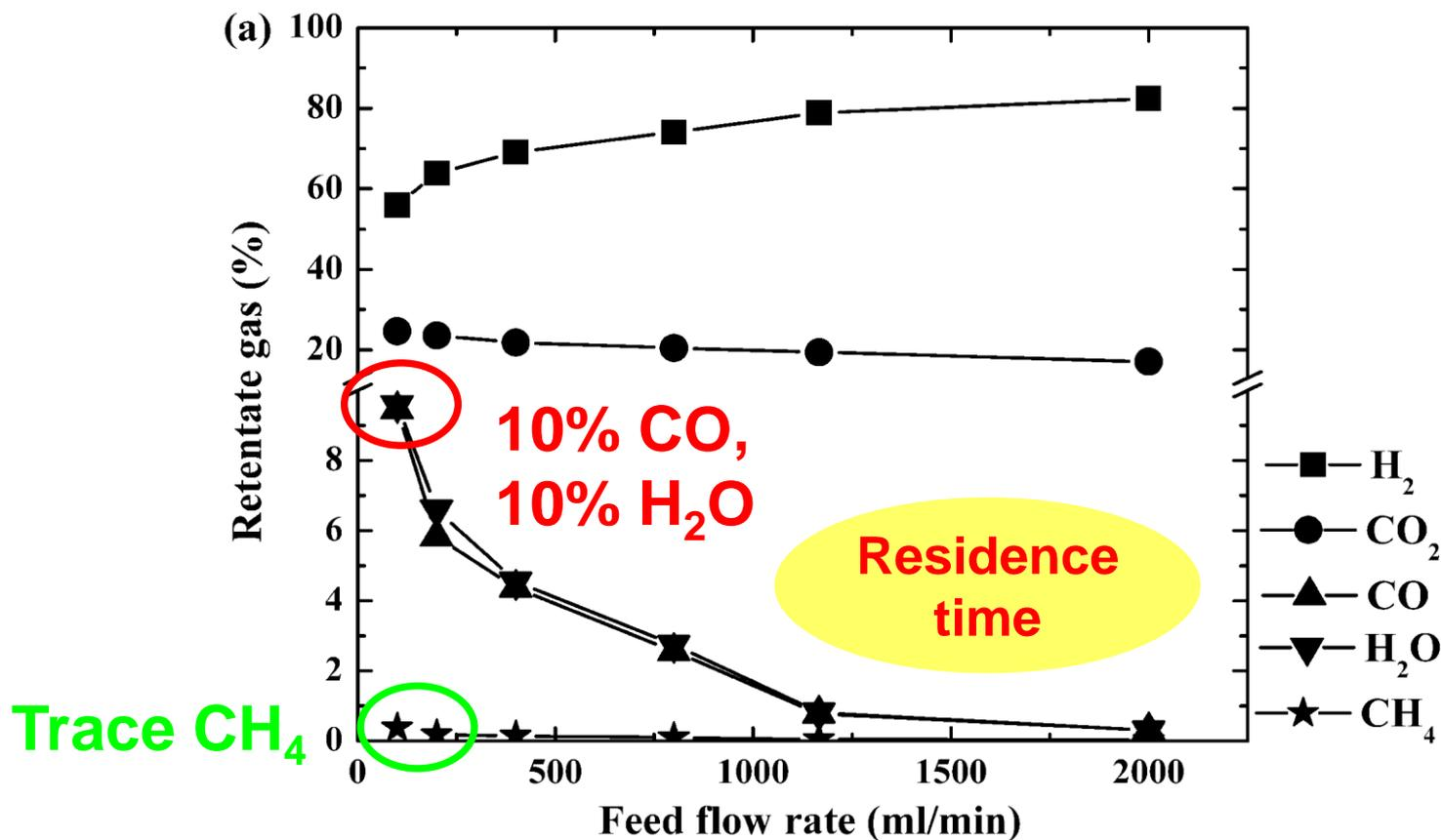
10% CO<sub>2</sub>/H<sub>2</sub> mixtures at 450 °C and 2 bar(a)
