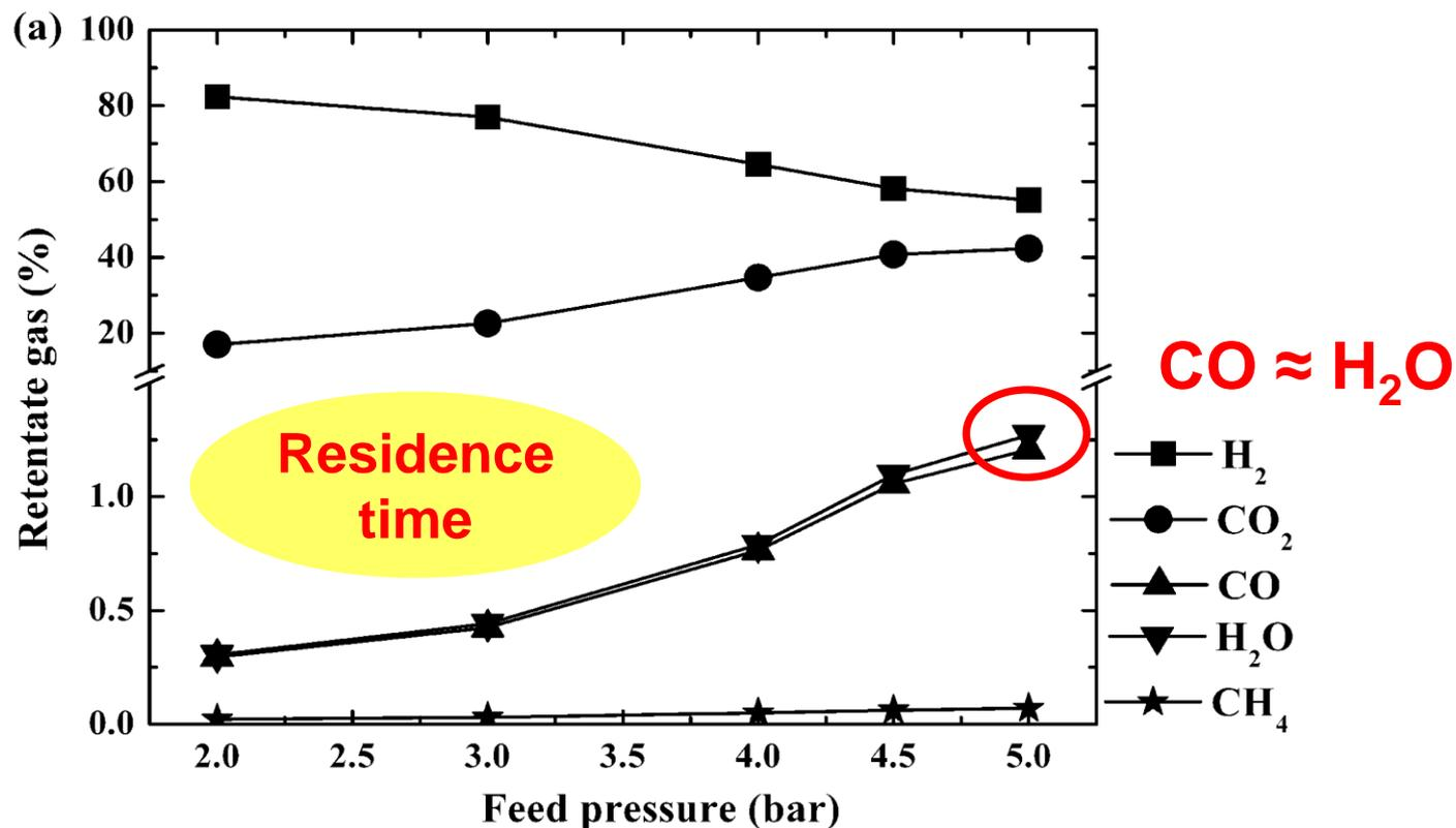
10%  $CO_2/H_2$  mixtures at 450 °C and a feed flow rate of 2 NI/min
