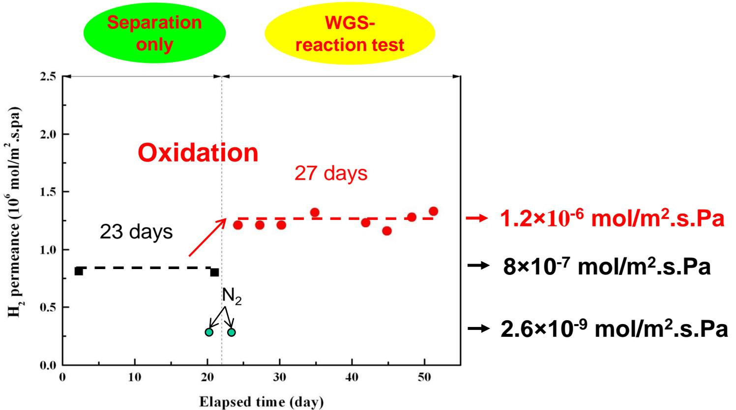
**N<sub>2</sub> permeance remained unchanged after catalyst loading**
