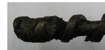
Molten lignin deposits at feed-screw tip
