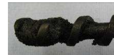
Molten lignin deposits at feed-screw tip
