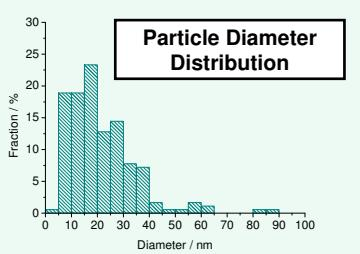
TEM results of a nickel steam-reforming catalyst prepared by impregnation on MgAl<sub>2</sub>O<sub>4</sub> support; EFTEM: three-window method, Ni L<sub>2,3</sub> edge; average diameter of Ni particles 21.4 nm.
