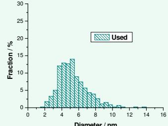
Pt catalyst particles on carbon support (Hispec 9100), top: before use, average diameter 2.4 nm, bottom: catalyst particles from used fuel cell cathode (30000 cycles between 0.7 and 0.9 V at 80 °C), average diameter 5.4 nm.
