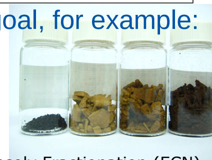
Lignin products from Modified Organosolv Fractionation (ECN)
