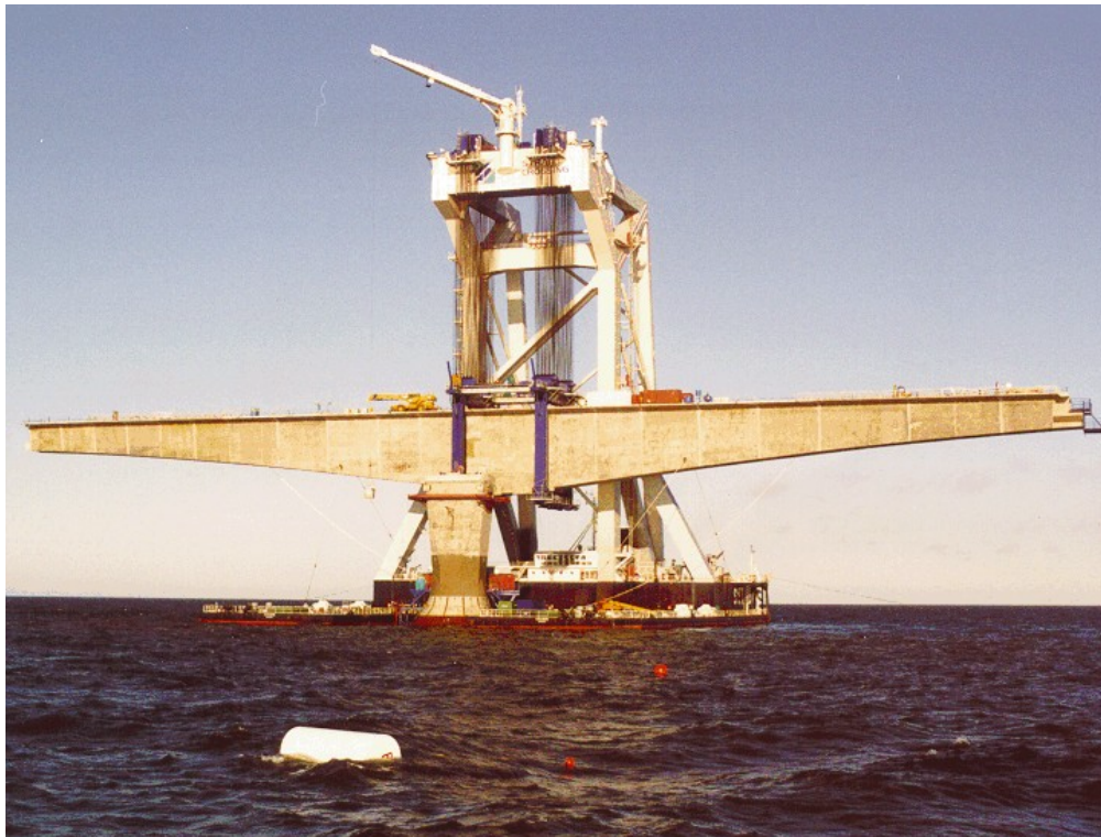
Figure 52. Very Heavy Lifting Vessel, The Svanen. The Svanen in action during the transport of a bridge piece. Courtesy: Ballast Nedam; http://www.ballast-nedam.nl .
