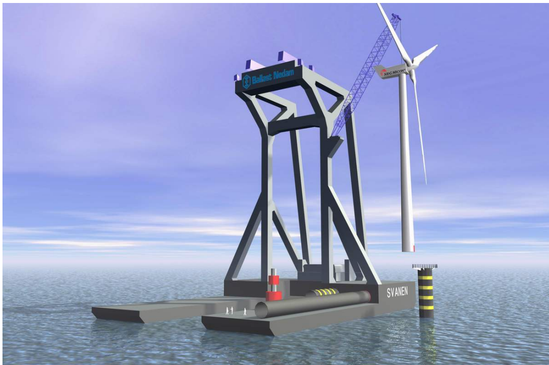
Figure 51. Very Heavy Lifting Vessel, The Svanen. Artist impression of the Svanen while installing a tower-nacelle-rotor assembly of a wind turbine on its support structure offshore. Courtesy: Ballast Nedam; http://www.ballast-nedam.nl .
