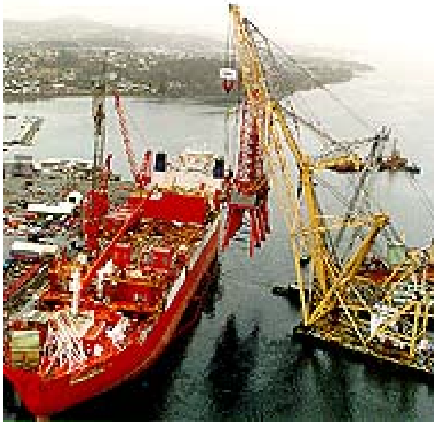
Figure 43. Typical Sheer Leg Vessels (right side of the picture). Source: Smit International; Internet site: http://www.smit.com
