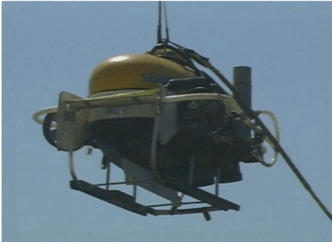
Figure 45. Typical Remote Operating Vehicle (ROV). Source: Van der Stoel Cable, Submarine Cable Installation Contractors; CD-Rom with company profile, version 01-08-2000
