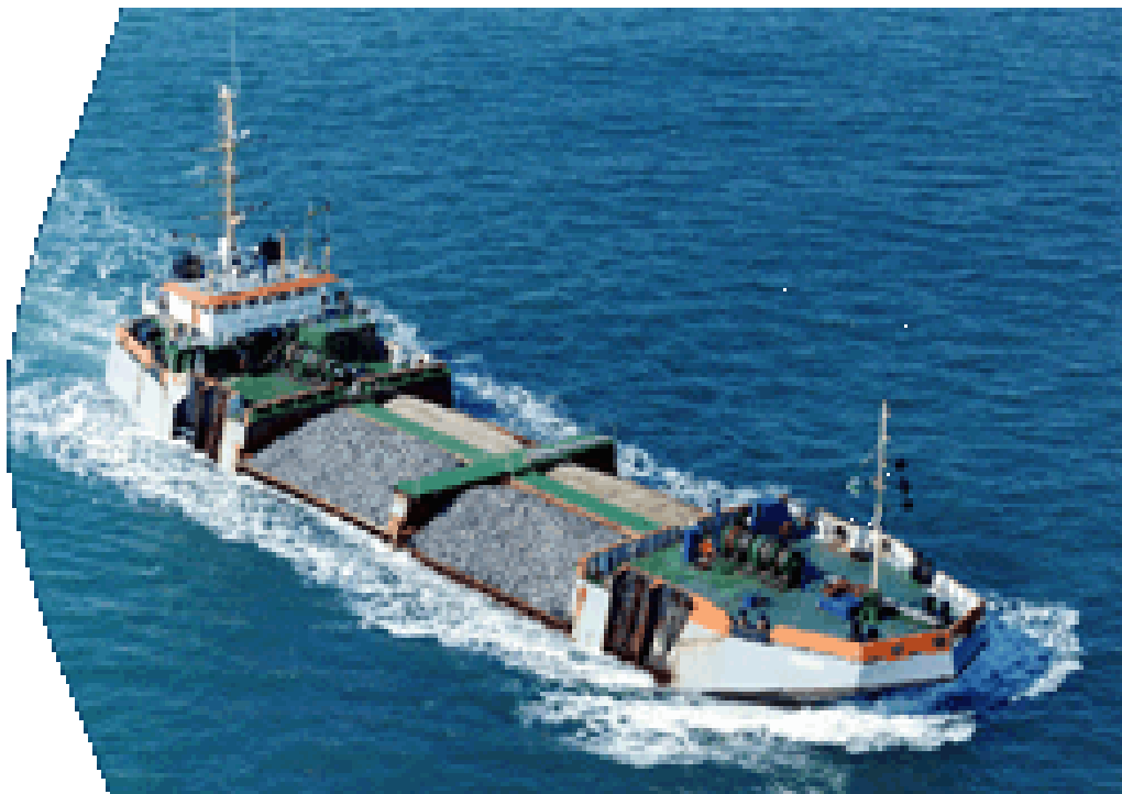
Figure 44. Typical Side Stone Vessel. Source: Van Oord ACZ; Internet site: http://www.vanoordacz.nl
