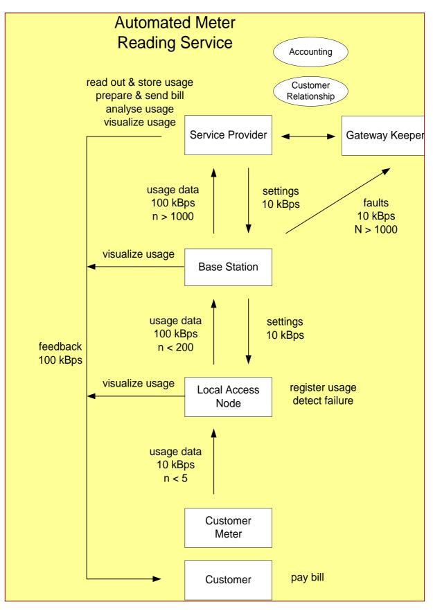
Figure 3.2. Powerline Automatic Meter Reading Schedule
