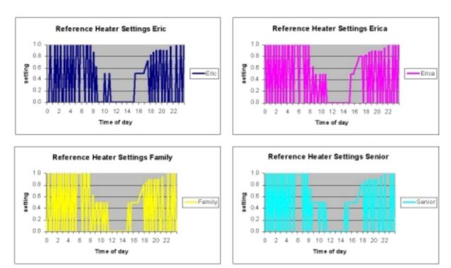
*Figure 6.2. Heater settings for the different winter scenarios in the reference situation*
