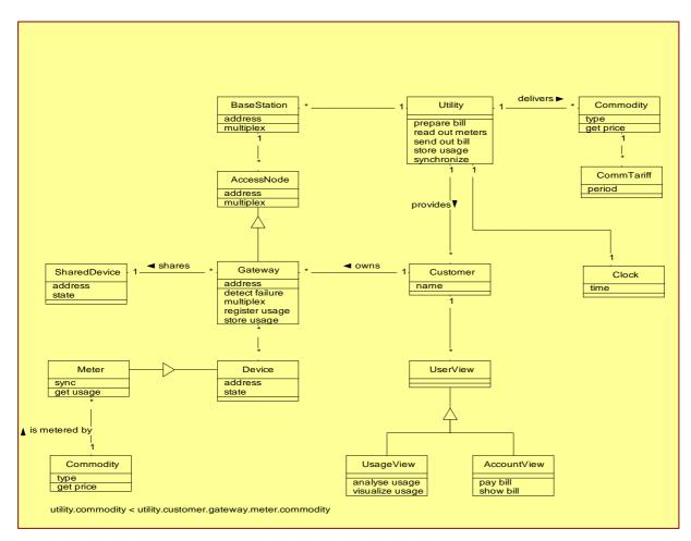
Figure 3.3. UML Object Diagram Automatic Meter Reading
