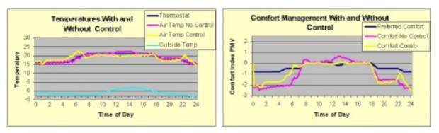
Figure 6.21. Left the initial and Comfy-controlled temperature progress for indoor air temperature; as a reference also the outdoor temperature and the thermostat settings are given. Right the initial and Comfy-controlled comfort; as a reference the preferred comfort is given.
