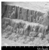
▲ Fig. 1 & 2: The material consists of small silicon columns. The spacing between the columns accommodates the volume expansion during lithiation and prevents cracking of the anode. In the most recent experiments (right picture) it has been demonstrated that it is possible to deposit thicker layers of 10u.
