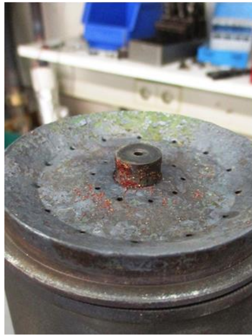
Figure 5. The ECN feeding system developed for high viscous liquids and the injection point located in the centre of the WOBs distributor plate (right).
