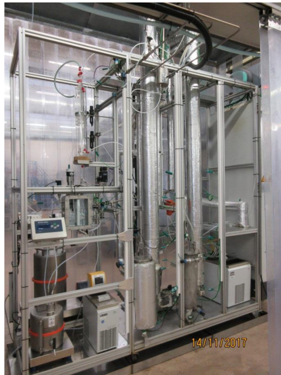
Figure 12. Upgraded BTX scrubbing unit, including new AWOS setup.
