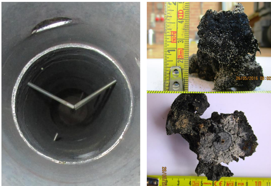
Figure 8. Internal view of the reactor and the unconverted humins-char agglomerate obtained during the humins gasification tests. Start bed temperature of 750°C.
