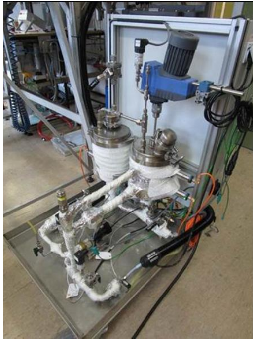
Figure 5. The ECN feeding system developed for high viscous liquids and the injection point located in the centre of the WOBs distributor plate (right).
