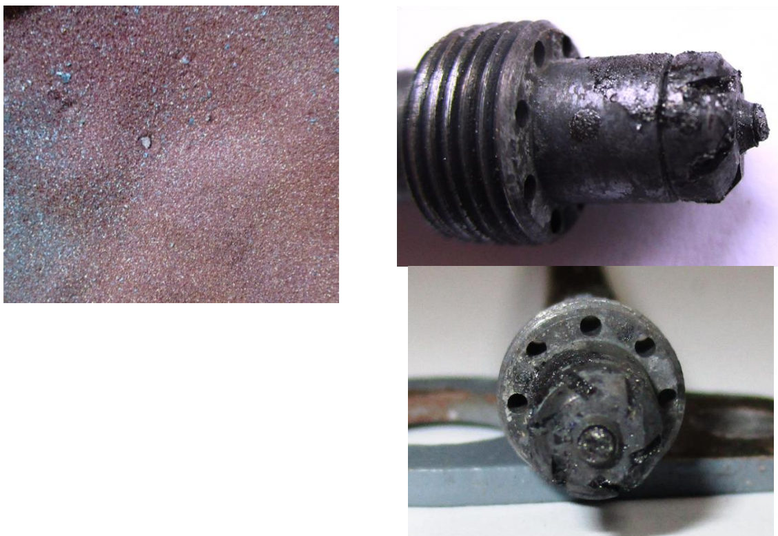
Figure 11. View of the bed material and the humins injection probe tip after the combustion test with humins.
