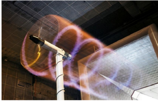
Figure 5.1: The MEXICO rotor in the DNW wind tunnel (left) and the CAD model of the of the rotor with blade 2 off-pitched (right).
