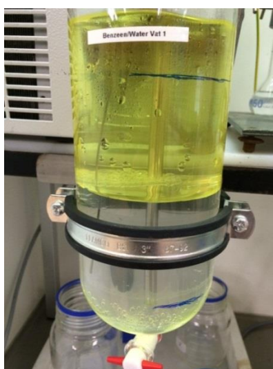
Figure 15 Bio-BTX recovery during tests in November 2014. The upper yellow layer corresponds to bio-BTX, the lower layer is condensed water from the stripper.
