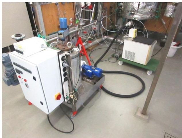
Figure 6 Setup for feeding of humins to the MILENA gasifier.
