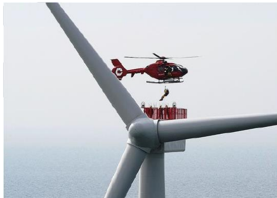
Figure 7: A helicopter transporting a technician to a wind turbine [20]
