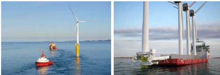
Figure 9: Example of towing vessels
