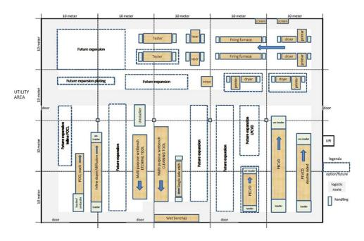
Figure 8: Proposed Floorplan for PV cell laboratory
