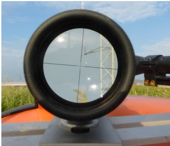
Figure 6: Theodolite pointing at the sonic anemometer during white box calibration.
