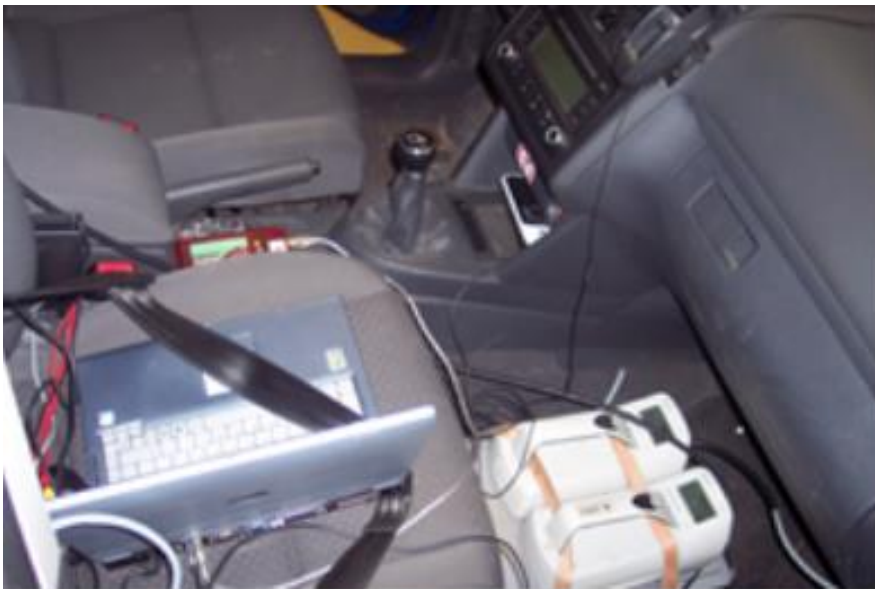
Figure 2: The two NO x monitors and computers logging the data
