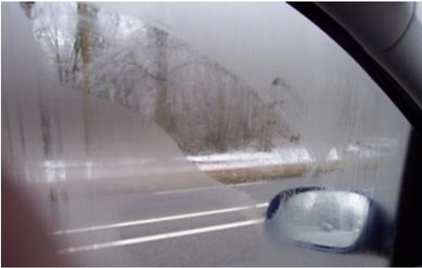
Figure 12: Windows in a car fogged up due to lack of ventilation
