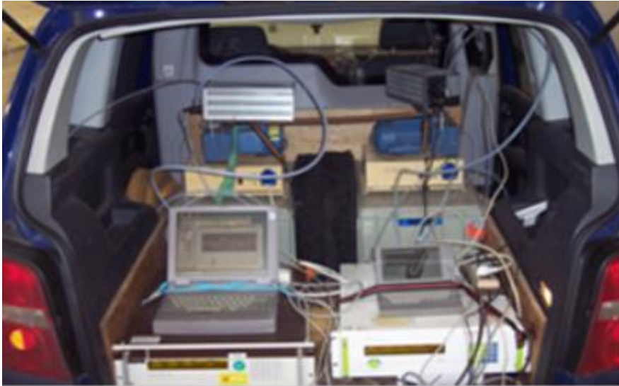
Figure 2: The two NO x monitors and computers logging the data
