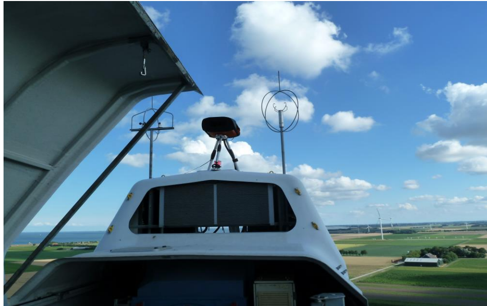
Figure 1: Wind Iris mounted on the back of the nacelle of test turbine N6.
