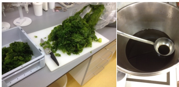
Figure 9-8 Ulva feedstock (left) and process product from hydrolysis at 140 °C (run 1, right).
