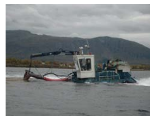
d) Vessel with a vaccum-sucker, used to harvest Ascophyllum nodosum in Norway © Rebours.
