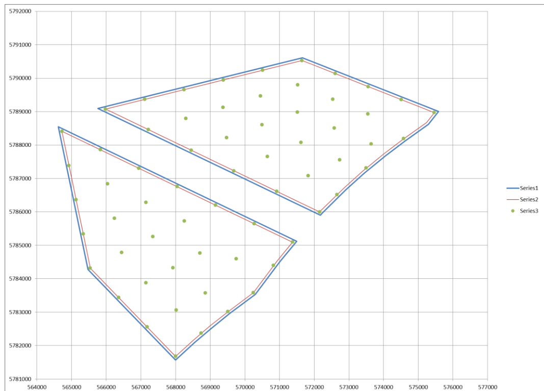
Figure 10: The lay-out of Site III with 6 MW wind turbines
