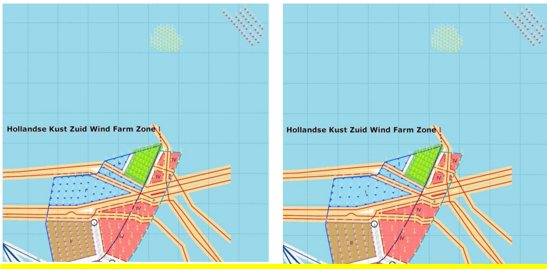
Figure 3: The HKZ wind farms, enclosing OWF Luchterduinen and showing the location of the OWF Prinses Amalia (yellow) and OWEZ, on the left the HKZ with 6 MW wind turbines and on the right with 8 MW wind turbines.
