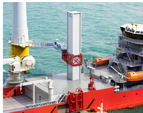
Figure 21: Barge Master Gangway [27].
