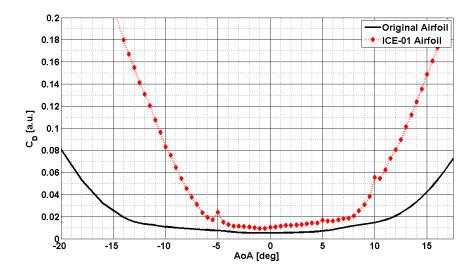
Figure 19: Comparison of Clean and Iced (ICE-01) Drag Characteristic  $C_D(AoA)$  for the NACA63418 Airfoil
