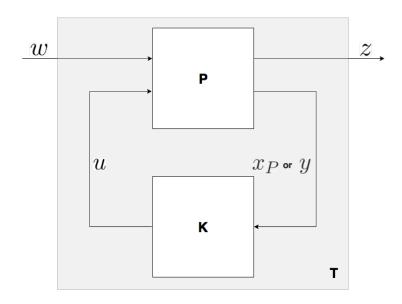
Figure 51: Generalized Feedback Interconnection (LFT)
