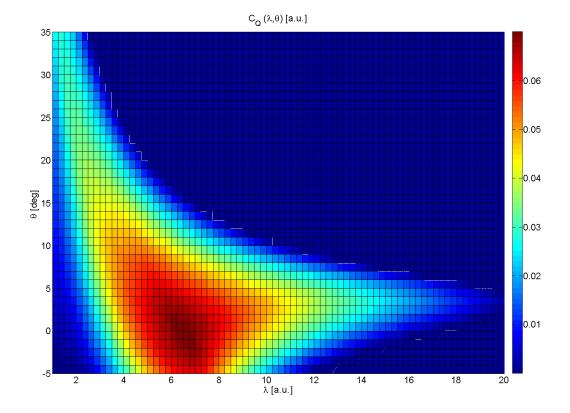
Figure 9: Rotor Torque Coefficient Curve for the ART 5 MW
