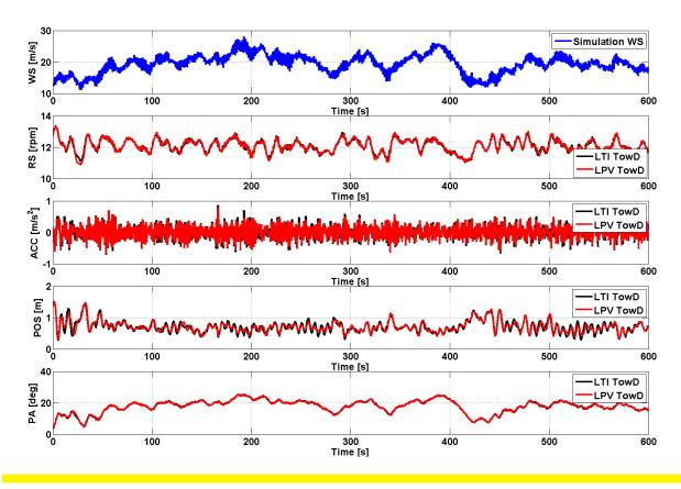
Figure 48: Time Series Comparison for Full-Load Conditions with Nominal and Off-Spec (-20% in NF) Tower for the ART 5 MW
