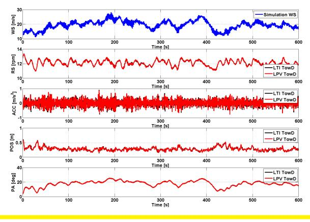
Figure 50: Time Series Comparison for Full-Load Conditions with Nominal and Off-Spec ( $\pm 20\%$  in NF) Tower for the ART 5 MW
