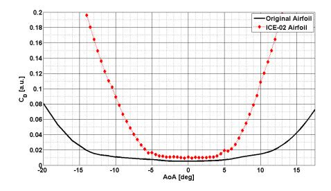
Figure 26: Comparison of Clean and Iced (ICE-02) Drag Characteristic  $C_D(AoA)$  for the NACA63418 Airfoil
