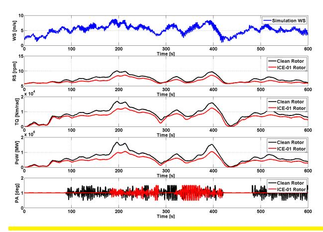
Figure 23: Time Series Simulation for Partial-Load Conditions with Clean and Iced (ICE-01) Rotor for the ART 5 MW
