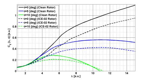
Figure 28: Comparison of Clean and Iced (ICE-02) Rotor Thrust Coefficient Curves  $C_T(\lambda, \theta)$  for the ART 5 MW Rotor
