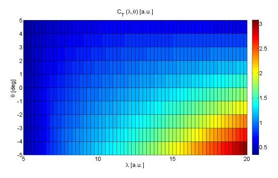
Figure 8: Rotor Thrust Coefficient Curve for the ART 5 MW
