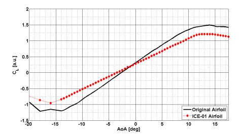
Figure 18: Comparison of Clean and Iced (ICE-01) Lift Characteristic  $C_L(AoA)$  for the NACA63418 Airfoil
