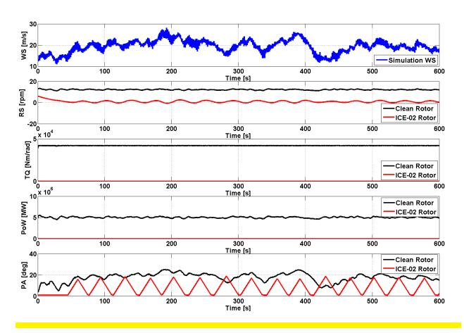
Figure 31: Time Series Simulation for Full-Load Conditions with Clean and Iced (ICE-02) Rotor for the ART 5 MW
