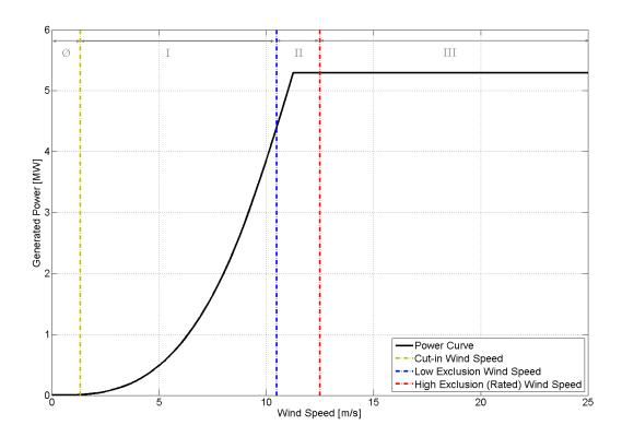
Figure 12: Power Curve and Possible Operation Regions for the ART 5 MW
