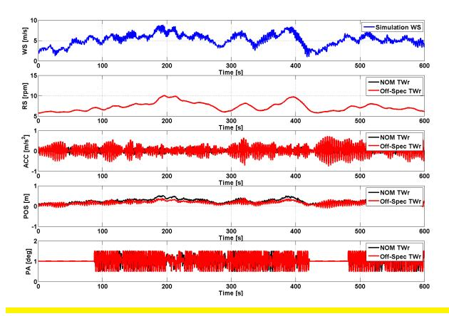
Figure 38: Time Series Simulation for Partial-Load Conditions with Nominal and Off-Spec (+20% in NF) Tower for the ART 5 MW
