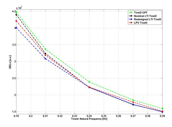
Figure 46: DEL Comparison for the ART 5 MW for Above-Rated Simulations with Different Active Tower Damping Controllers
