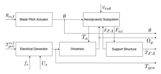
Figure 7: Main Subsystems within a Wind Turbine
