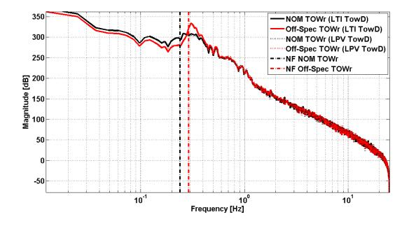
**Figure 44:** Comparative Spectra of Tower Bottom Moment based on Partial-Load Simulation of the ART 5 MW with Nominal and Off-Spec (+20% in NF) Support Structure
