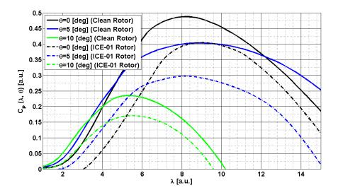
**Figure 20:** Comparison of Clean and Iced (ICE-01) Rotor Power Coefficient Curves  $C_P(\lambda,\theta)$  for the ART 5 MW Rotor
