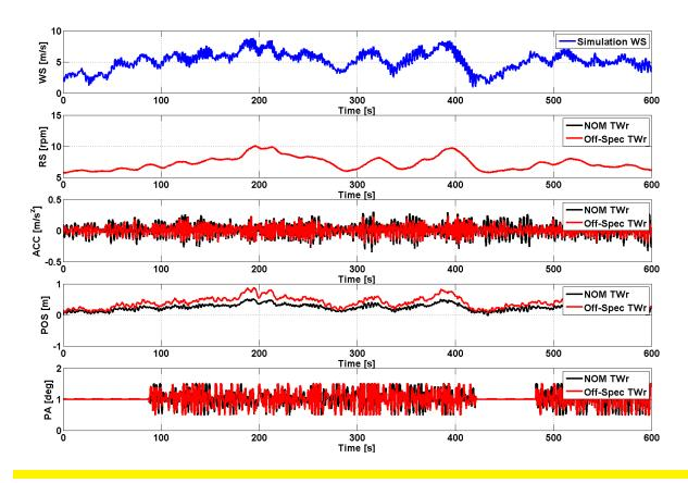
Figure 36: Time Series Simulation for Partial-Load Conditions with Nominal and Off-Spec (-20% in NF) Tower for the ART 5 MW
