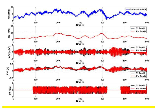
Figure 49: Time Series Comparison for Partial-Load Conditions with Nominal and Off-Spec (+20% in NF) Tower for the ART 5 MW
