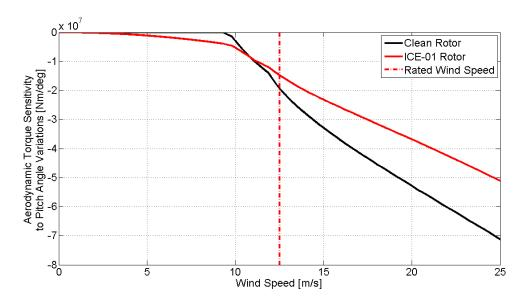
Figure 22: Aerodynamic Torque Derivatives with respect to Pitch Angle for the Clean and the Iced (ICE-01) Rotor of the ART 5 MW
