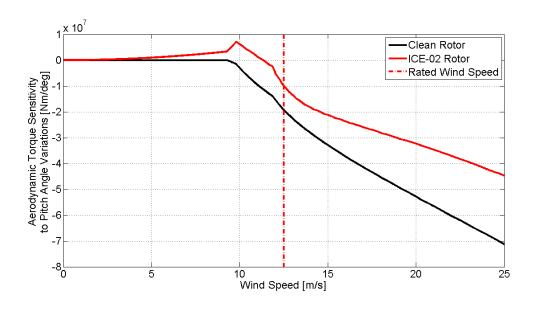
Figure 29: Aerodynamic Torque Derivatives with respect to Pitch Angle for the Clean and the Iced (ICE-02) Rotor of the ART 5 MW
