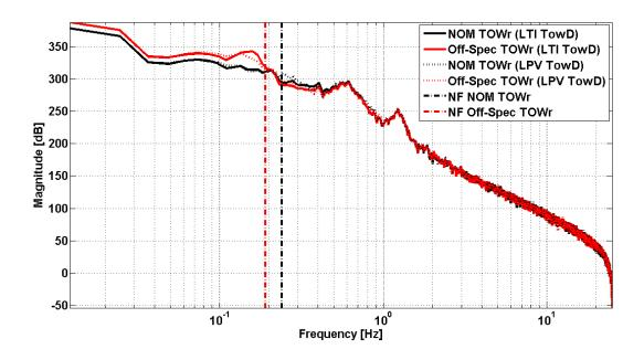
Figure 43: Comparative Spectra of Tower Bottom Moment based on Full-Load Simulation of the ART 5 MW with Nominal and Off-Spec (-20% in NF) Support Structure
