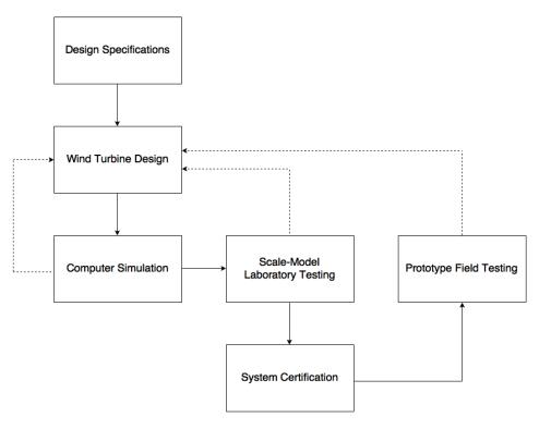
Figure 14: Overview of the Wind Turbine Design and Certification Process
