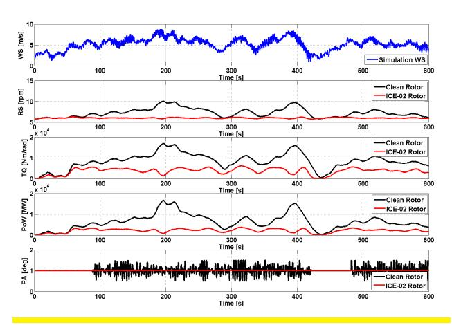
Figure 30: Time Series Simulation for Partial-Load Conditions with Clean and Iced (ICE-02) Rotor for the ART 5 MW
