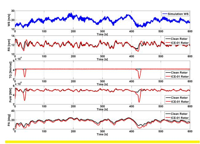
Figure 24: Time Series Simulation for Full-Load Conditions with Clean and Iced (ICE-01) Rotor for the ART 5 MW
