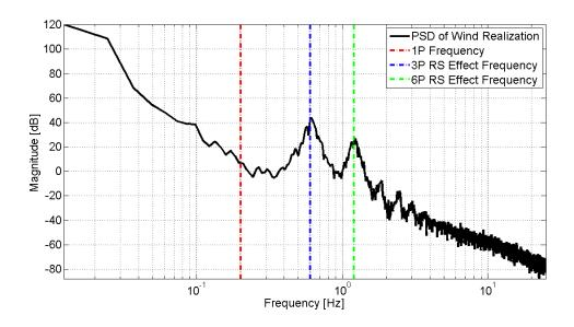
Figure 6: Power Spectrum of a Rotor-Effective Wind Realization for the ART 5 MW
