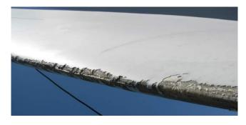
Figure 15: Ice Accretion on a Turbine Rotor
