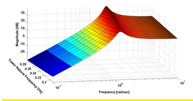
**Figure 40:** Magnitude Bode Plot of the  $\delta \theta(t) o \delta \ddot{x}_{FA}(t)$  Transfer from (4.1) for the Considered Range of Tower Natural Frequencies
