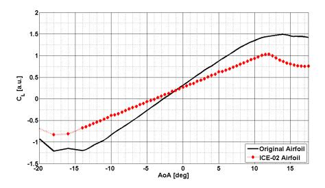
Figure 25: Comparison of Clean and Iced (ICE-02) Lift Characteristic  $C_L(AoA)$  for the NACA63418 Airfoil
