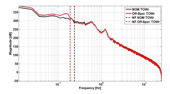
Figure 34: Spectra of Tower Bottom Moment based on Full-Load Simulation of the ART 5 MW with Nominal and Off-Spec (+20% in NF) Support Structure
