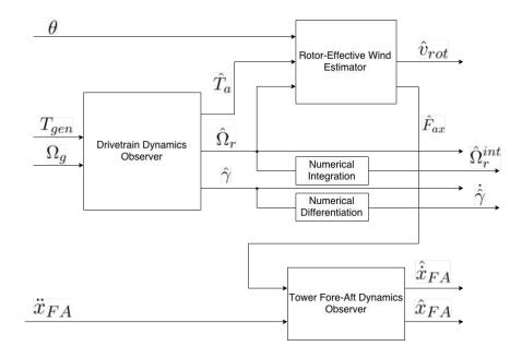
Figure 11: Overview of the Required Wind Turbine Information Reconstruction Algorithms
