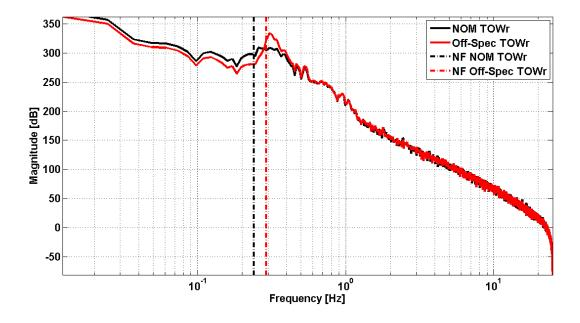
Figure 35: Spectra of Tower Bottom Moment based on Partial-Load Simulation of the ART 5 MW with Nominal and Off-Spec (+20% in NF) Support Structure
