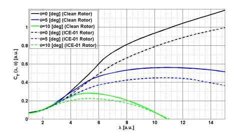
Figure 21: Comparison of Clean and Iced (ICE-01) Rotor Thrust Coefficient Curves  $C_T(\lambda,\theta)$  for the ART 5 MW Rotor
