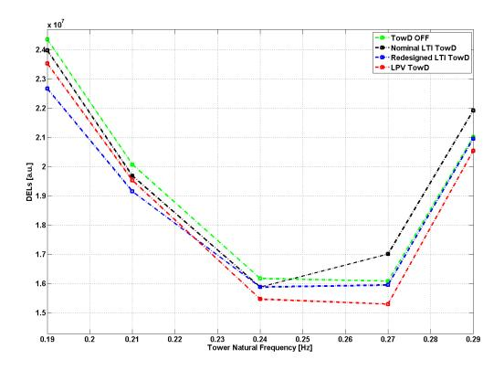
Figure 45: DEL Comparison for the ART 5 MW for Below-Rated Simulations with Different Active Tower Damping Controllers
