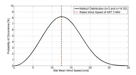
Figure 5: Fictitious Weibull Mean Wind Speed Distribution of a Potential Site for the ART 5 MW
