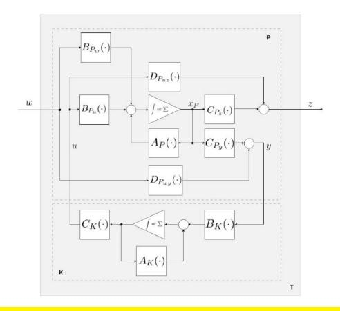
Figure 52: LFT Interconnection for  $\mathcal{H}_2$  Dynamic Output-Feedback Control
