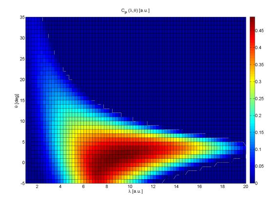
Figure 10: Rotor Power Coefficient Curve for the ART 5 MW
