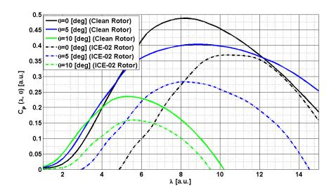
**Figure 27:** Comparison of Clean and Iced (ICE-02) Rotor Power Coefficient Curves  $C_T(\lambda, \theta)$  for the ART 5 MW Rotor
