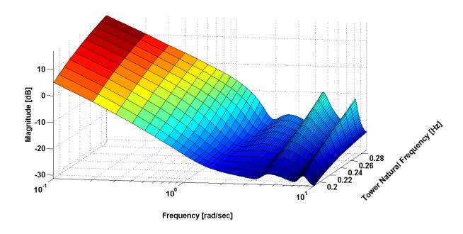
**Figure 41:** Magnitude Bode Plot of the  $\delta\ddot{x}_{FA}(k) \to \delta\theta(k)$  Transfer of the LPV Tower Damping Controller for the Considered Range of Tower Natural Frequencies
