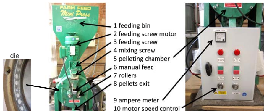
Figure 43: Lab scale ring die pellet mill
