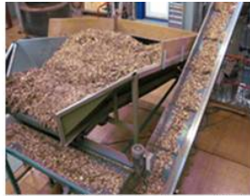
Chips are fed via bunker and belts
