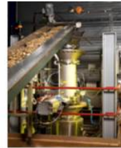
Lock hopper on top of the reactor
