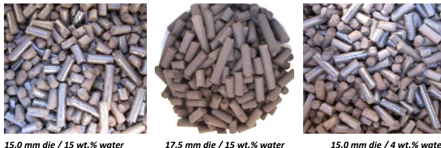
Figure 46: Pellets from torrefied bamboo (tests I to K)
