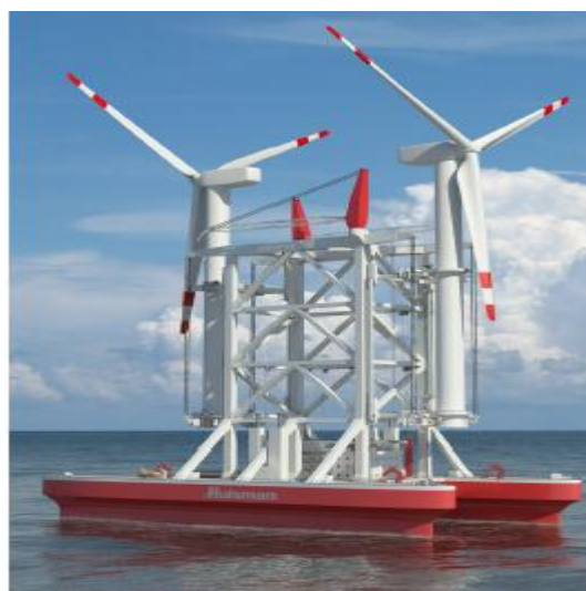
Figure 25: Huisman Shuttle vessel with a capability of single lift installation of turbines [15]
