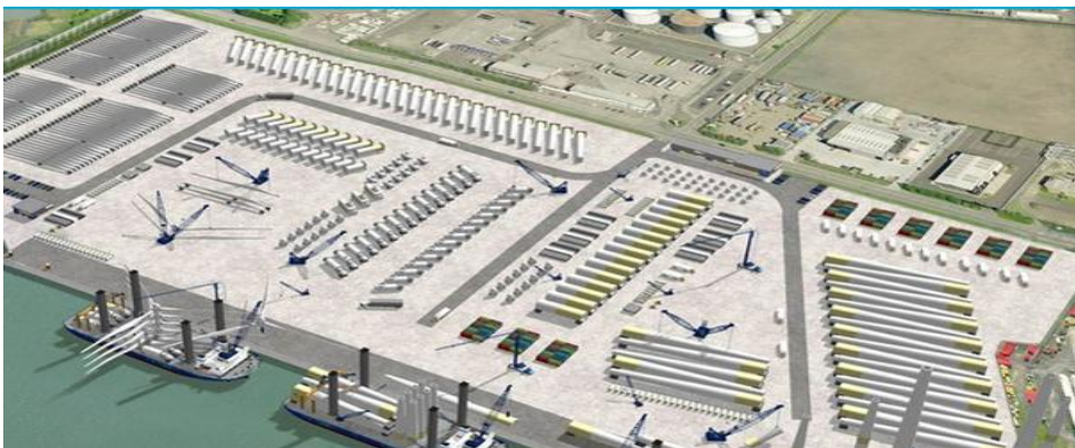
Figure 23: Example of an onshore harbour with different components placed for installation [13]
