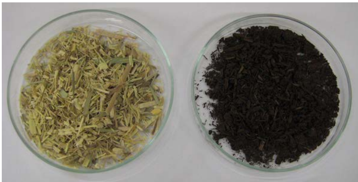
Figure 6 Raw Arundo donax (left) and Arundo donax after TORWASH (right)
