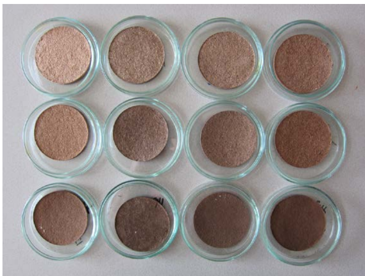
Figure 3 Pressed discs of (from left to right) Miscanthus, Fibre sorghum, Triticale and Arundo donax, with the lowest temperature at the top and highest temperature at the bottom
